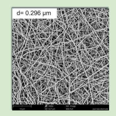
Very thin fibers can be formed (with diameter below 1 µm).
