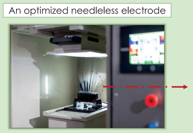
The needleless emitter/spinneret allows for multiple Taylor cone formation, many particles/fibers can be fabricated, increasing the productivity of the electrospraying/electrospinning process.
